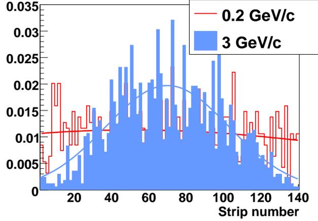
Figure 4: Distribution of the hit position in the most upstream detector using 3 GeV/c (full) and 0.2 GeV/c (hollow)  $\pi^-$  beam. The two curves are gaussian fits.
