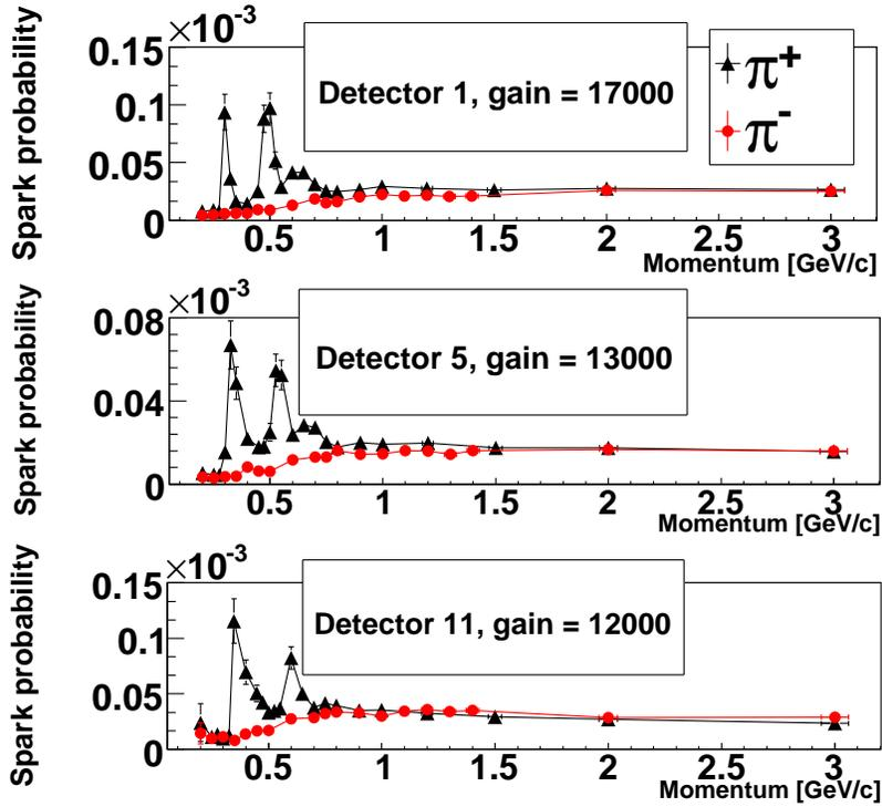
Figure 6: Discharge probability as a function of the beam momentum for  $\pi^-$  (circles) and  $\pi^+$  (triangles) for detectors in position 1, 5 and 11. Statistical and systematic errors (from the luminosity correction factor) are included.
