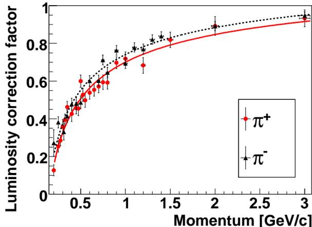
Figure 5: Luminosity correction factor (C) for one detector, as a function of the beam momentum, calculated with  $\pi^+$  and  $\pi^-$  data. The curves are fits of the form  $\alpha + \beta/p^{0.4}$ .
