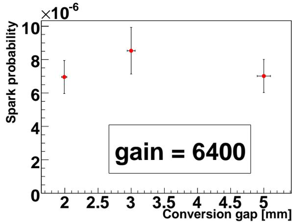
Figure 7: Discharge probability as a function of the conversion gap height for 3 GeV/c  $\pi^-$  beam. Statistical and systematic errors are included.
