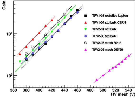
Figure 2: Gains measured as a function of the micro-mesh high voltage for some of the non GEM detectors. The detector with the smallest gains has a thicker micro-mesh and a 192 micron amplification gap.
