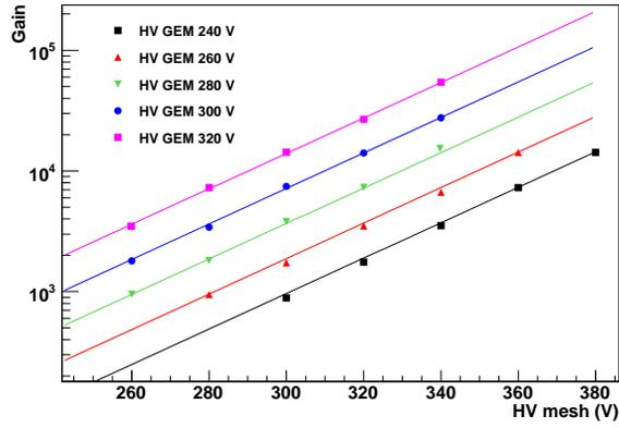
Figure 3: Gains as a function of the micro-mesh high voltage for the MMGEM with a 2 mm transfer gap. The transfer field is 100 V/mm and the GEM high voltage is varied from 240 V to 320 V.
