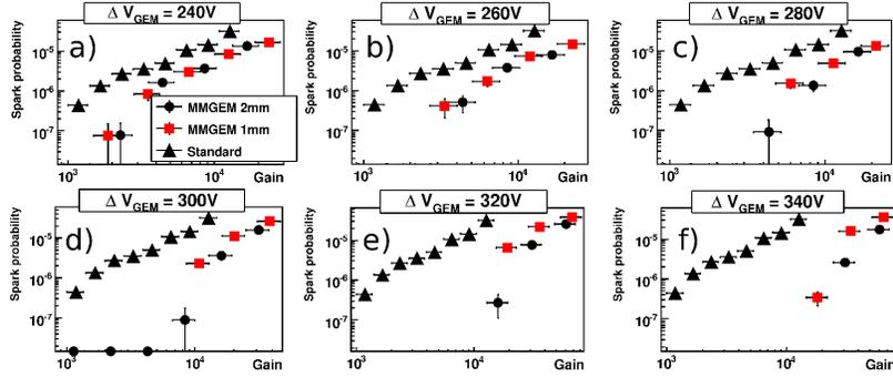
Figure 8: Discharge probability as a function of the total gain for the two MMGEMs and a standard Micromegas with 3 GeV/c  $\pi^-$ . From a) to f) the GEM high voltage is increased by steps of 20 V, with a constant transfer field of 300 V/mm for the two MMGEMs.
