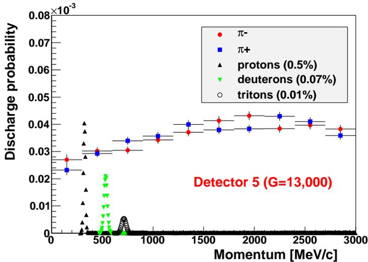
Figure 9: Geant4 simulation of the discharge probability as a function of the beam momentum obtained for different particles, in the detector 5 (with a gain of 13,000). Protons, deuterons and tritons are scaled to represent 0.5%, 0.07% and 0.01% of the  $\pi^+$  beam, respectively.
