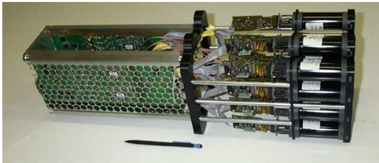
**Figure 3.5:** Photography of a H.E.S.S. camera drawer. The PMTs can be seen on the right. Ref. [61].
