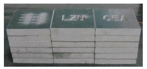
Figure 8-8. Polyethylene masks used for the neutron imaging.
