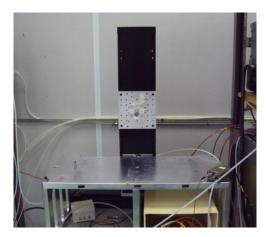
Figure 4-2. The set of two mechanical arms which holds the <sup>55</sup>Fe source.
