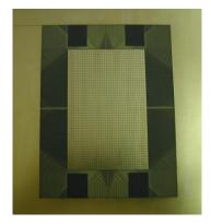
Figure 8-2. The PCB of the neutron detector (sensitive area:  $57.4 \text{ mm} \times 88.6 \text{ mm}$ ).
