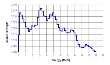
Figure 8-5. <sup>241</sup>Am-<sup>9</sup>Be source spectrum according to ISO 8529 standard.
