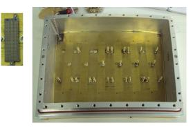
Figure 4-7. Mechanical problem: some studs de-soldered.
