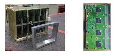
Figure 3-17. The T2K electronics. (a) the packaging of electronics for one module test; (b) one FEC (14 cm  $\times$  25 cm ).
