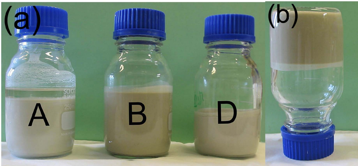
Figure 2. (a) dispersions of clays after 12 hours at rest and (b) illustration of the thixotropic behavior of some samples (sample D).
