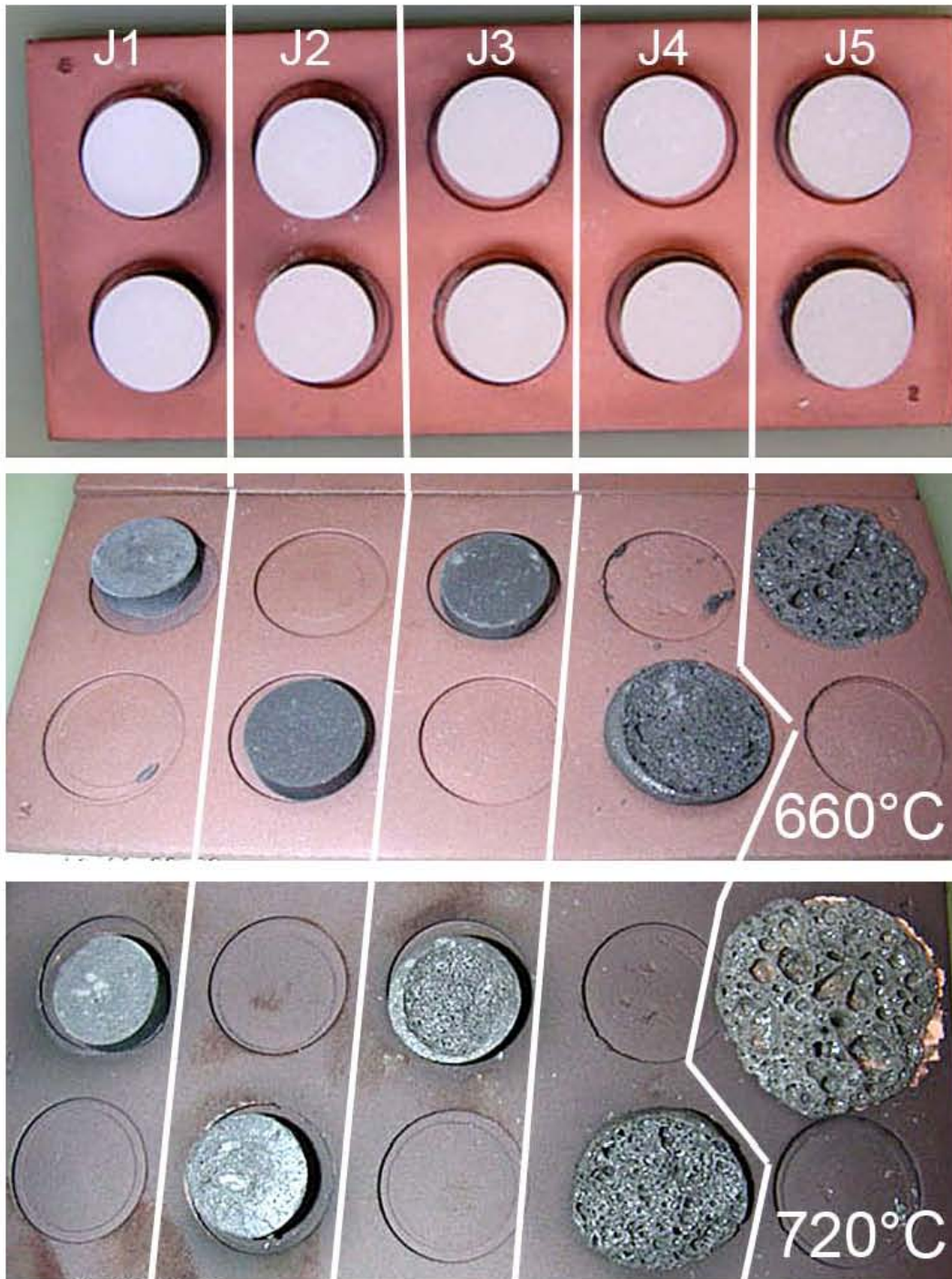
Figure S13: Evolution of the ceramic pellets as a function of the thermal treatment. From top to bottom: as-prepared, 600°C, 720°C. See Table II for compositions
