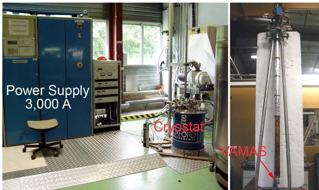
Figure S4: (left) Cétacés power station for the measurement of superconductors under a high magnetic field and at low temperature; (b) close view of the measurement stick that is inserted into the cryostat: the VAMAS sample is located at the bottom and the electrical current is provided by an over-dimensioned copper stick to avoid any Joule effect.
