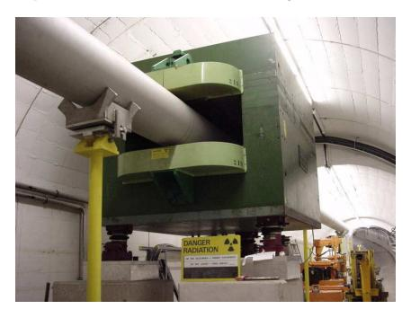
Figure 3.5: The dipole magnet sweeps the charged particles off the beam.
