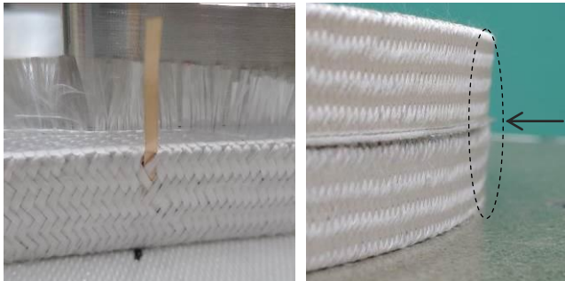
Fig. 6. Details of the coil: a) voltage tap; b) close-up on the ends.
