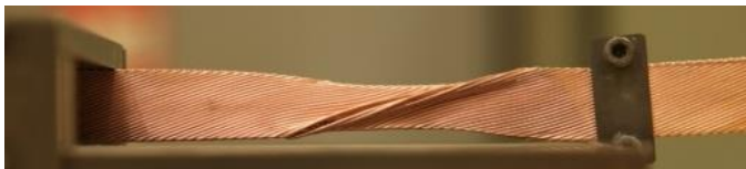
Fig. 3. Unsupported cable end collapsed due to the tension generated during heat treatment without gaps in the mandrel.
