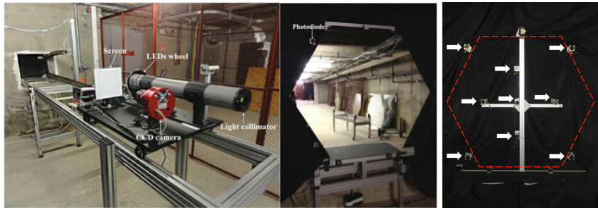
Figure 3.7: Left : Optical table. Center : Mirror support. Right : Photodiodes attached to the mirror support (5 of them are behind the mirror for background monitoring and for light pool uniformity measurement.).
