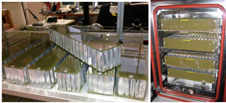
Figure 3.11: Left : Small samples of 100 mm by 50 mm by 80 mm with a curvature radius of 30 m. Right : Samples inside the climate chamber.
