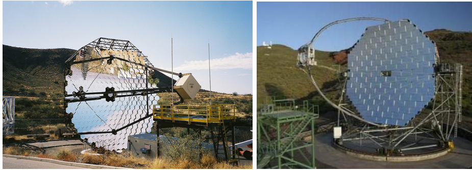
Figure 3.1: Telescopes of the VERITAS array (left) and the MAGIC array (right). The reflectors of these telescopes are composed by small mirror facets.
