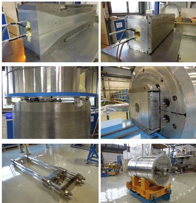
Fig. 2. Components of the FRESCA2 support structure. Up-left: dummy coils and vertical pads. Up-right: the coil-pack composed of dummy coils and vertical and horizontal pads. Center-left: the shell sliding around the two
