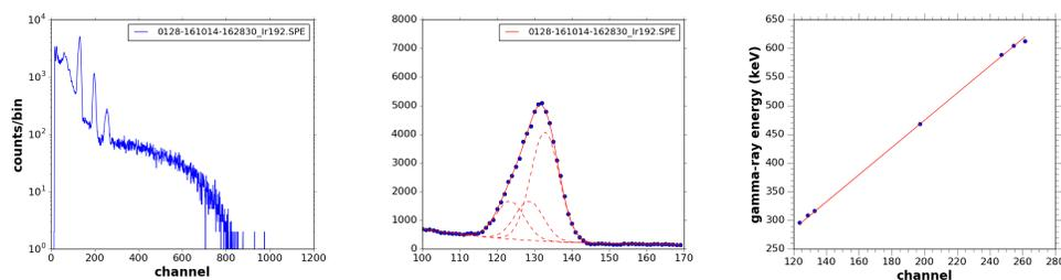
**Figure 3:** The measured spectrum of the  $^{192}\text{Ir}$  source (left panel), a zoom on the first triplet together with the fitted Gaussians with a fixed ratio of intensities (middle panel), and the resulting channel to energy calibration (right panel).
