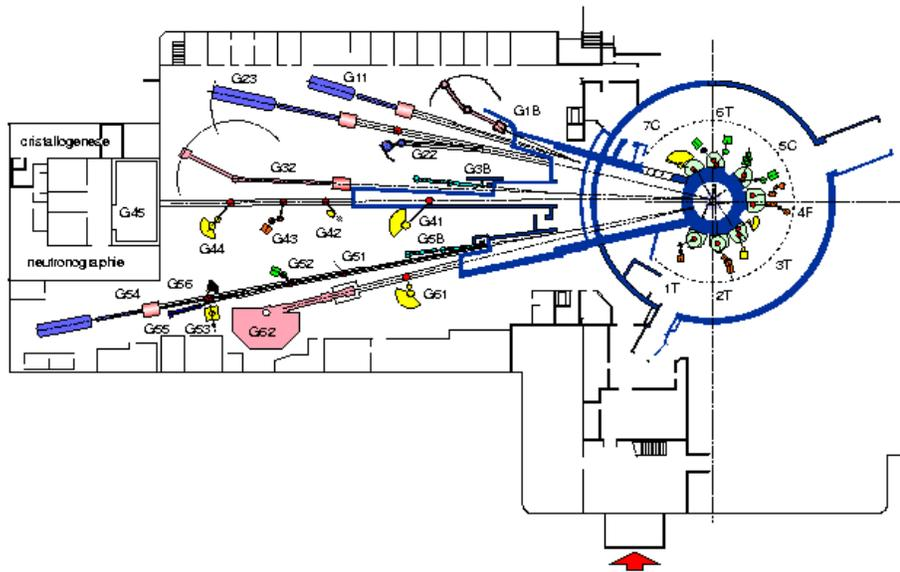
**Figure 1:** The layout of the neutron beam lines of the reactor Orphée [1,4]. Experimental area G4-3 was used for the boron determination experiment.
