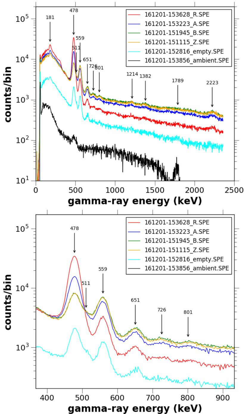
**Figure 4:** The measured spectra of all samples, corresponding to an irradiation time of 180 seconds, shown as the full energy region (upper panel) and a zoom in the region containing the 478 keV peak from boron (lower panel).
