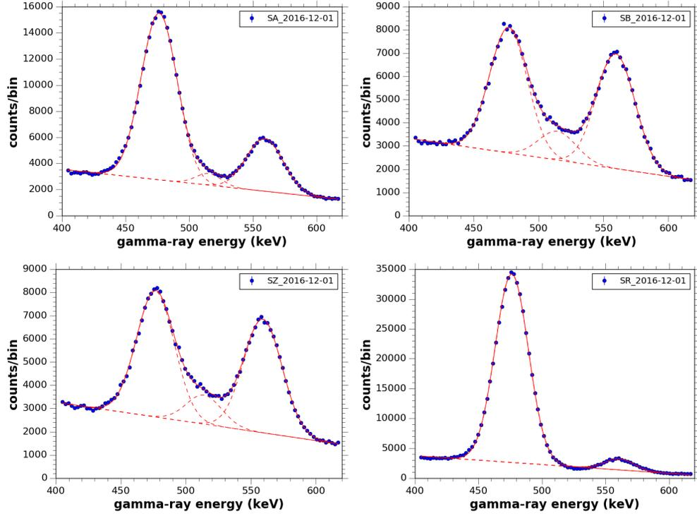
**Figure 5:** A zoom of the measured spectra in the region of the 478 keV peak together with a fit of three gamma-rays from which the peak areas are determined, for each of the four samples A, B, Z, and R.
