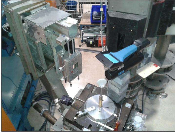
**Figure 2:** One of the tested setups for the measurement. A white polyethylene sample is positioned in the neutron beam, shape by the final borated aluminum collimator. For the final measurement, the distance of the standalone Iris CeBr<sub>3</sub> detector system was with respect to the sample was increased.
