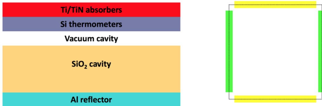
FIGURE 3.12: Left : Stack of the different layers defining the \lambda/4 cavity (thicknesses : Si : 1.5 \mu\text{m} , vacuum cavity : 2 \mu\text{m} , SiO 2 cavity : 11 \mu\text{m} ). Right : The unit cell with four (half-) TiN absorbers, pattern seen from above the detector. The yellow and green dipoles correspond to the antennas (same color) of the figure 3.11, right.
