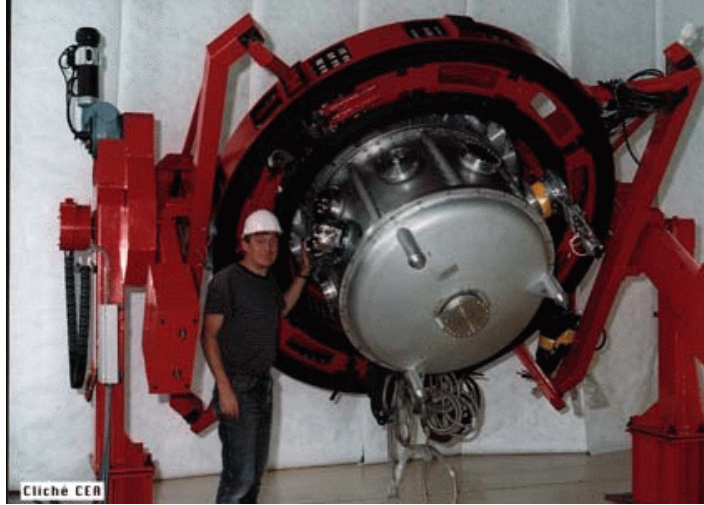
Fig. 1. Picture of the VISIR test cryostat and cable wrap mounted on the integration support.
