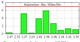
Figure 4 : Longitudinal impedances ( $k\Omega$ .GHz) versus monopole modes (frequency in GHz)
