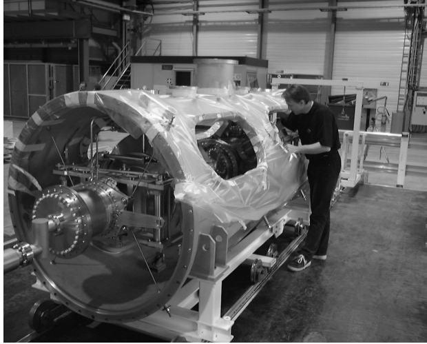
Figure 8: Preparation of the assembly before the mounting of the power couplers in the clean room.
