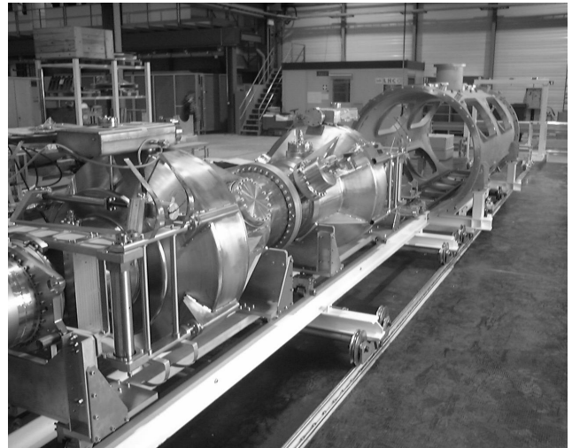
Figure 7: The two cavities in their helium tank and tuning systems before insertion into the vacuum vessel.
