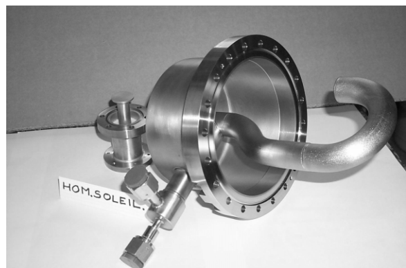
Figure 4: HOM coupler for monopole modes
