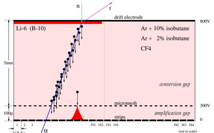
Figure 1: The Micromegas detector principle.
