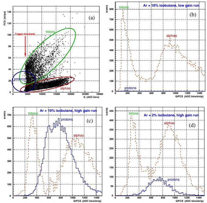
Figure 2: Fitted cluster size versus cluster charge (a) and  $Q/FCS$  distribution for proton recoils (solid line), tritons and alphas (dashed line) with (b) low gain, argon/isobutane (90:10), (c) high gain, argon/isobutane (90:10) and (d) high gain, argon/isobutane (98:2): In (b) no proton recoils are observed (cut by threshold), while from (c) to (d) the number of proton recoils drops according to the hydrogen concentration in the gas.
