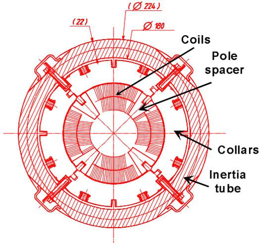
Fig. 1. Cross-sectional view of quadrupole magnet model.
