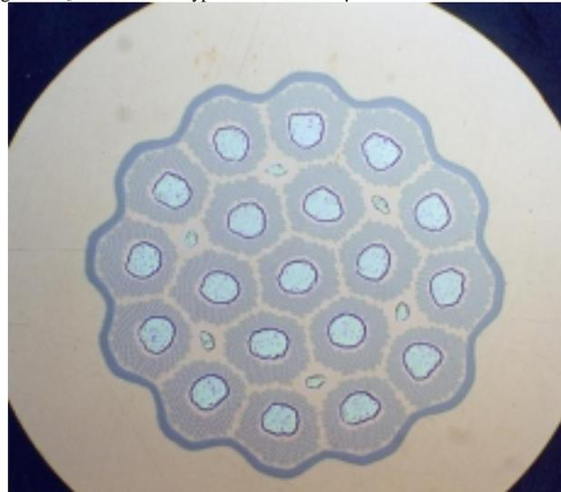
Fig. 4. Internal-tin strand layout developed by Alstom/MSA.
