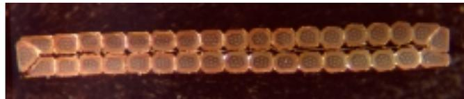
Fig. 3. Nb<sub>3</sub>Sn Rutherford-type cable with a 25- $\mu$ m-thick stainless steel core.
