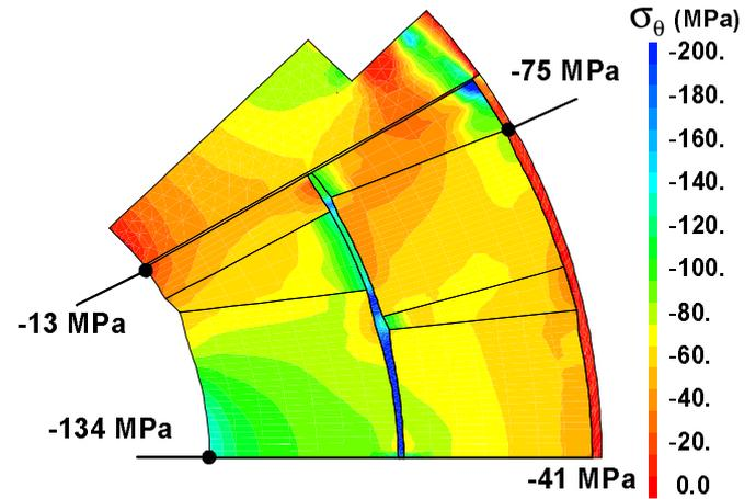
Fig. 2. Azimuthal coil stress distribution at 11,870 A.
