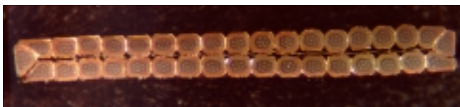
Fig. 2. Nb 3 Sn Rutherford-type cable with a 25- \mu m-thick stainless steel core.
