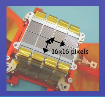
« CCD »-like filled bolometer array built by CEA for the PACS instrument on the ESA Herschel Space Observatory
