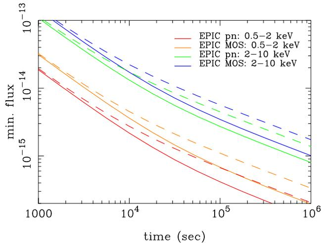
**Fig. 3.** EPIC sensitivity ( $5\sigma$  minimum detectable flux in erg cm $^{-2}$  s $^{-1}$  in respective bands) as a function of exposure time. Sensitivity is computed for an assumed  $\alpha = 1.7$  power-law spectrum with a column density  $N_H = 3 \times 10^{20}$  cm $^{-2}$ . Solid curves are for the nominal background rates quoted in the text. Dashed curves are for background levels enhanced by a factor 3. The EPIC MOS curves correspond to the combination of the two cameras.
