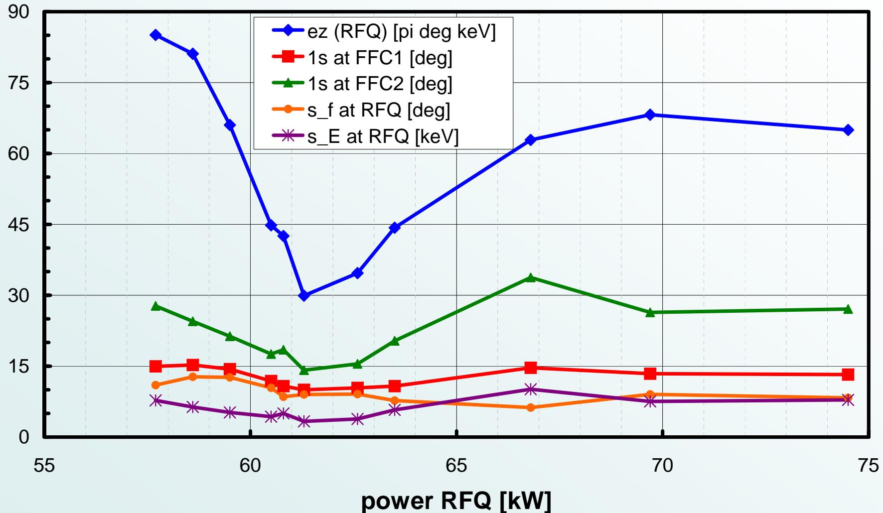
Specified longitudinal rms emittance =  $120 \pi$  deg keV, realistic value  $74 \pi$  deg keV
