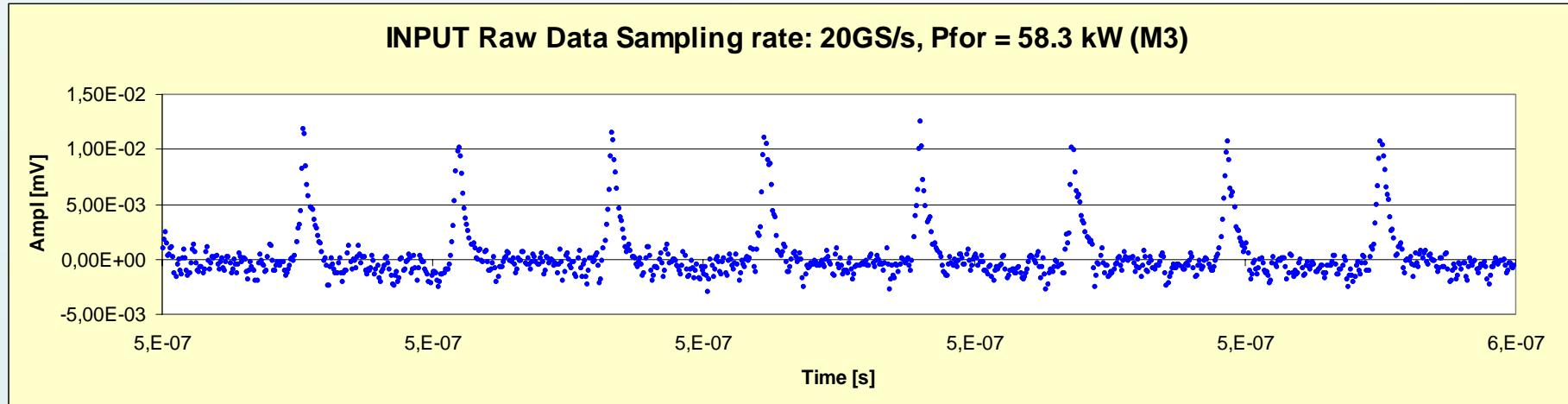
Measured longitudinal beam profile after averaging of up to 100 bunches of one macro-pulse and a Fourier correction.
