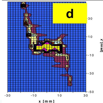
＼ If ions beam and neutral atoms beam are not concentric it points that lens is steering
