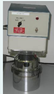
6" NaI detector Movable lead shield
