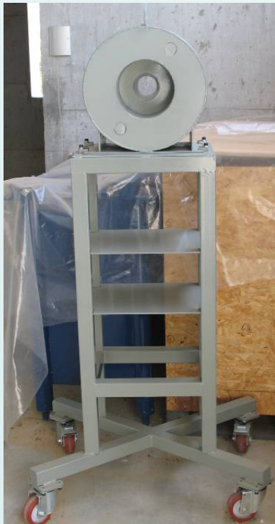
6" NaI detector Movable lead shield
