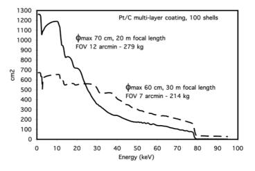
**Figure 2** : Mirror effective areas for two study cases. Both are assuming a multi-layer coating. Characteristics are given in the figure.
