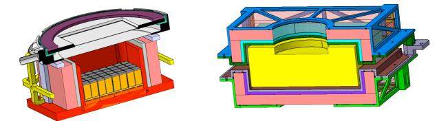
Figure 4 : sketch of the detector assembly. Left : internal detectors system, cut-view, with Macro-Pixel Detector on top, the array of Cd(Zn)Te modules at the bottom, and the active and passive shielding walls on the sides. Right : the internal detector system (central volume) is surrounded by additional active and passive shieldings, in two halves.
