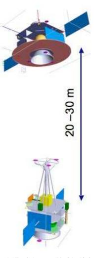
**Figure 1** : Sketch (not to scale) of the Simbol–X configuration in flight, with mirror (top) and detector (bottom) spacecraft kept on a constrained formation. The focal plane unit has a ~ 1.5 m collimator on top, while the mirror spacecraft carries a ~ 3 m diameter circular sky baffle (see Section 3.3).
