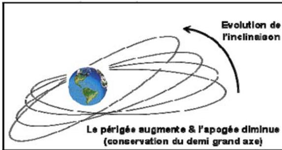
Typical operations on such an orbit consists in performing science during 6 days (out of perigee) and to use permanent perigee visibility to download the bigger part of the telemetry. Outside perigee a daily contact of one to two hours is sufficient for Status of Health and/or monitoring of the formation repointing to a new target.
