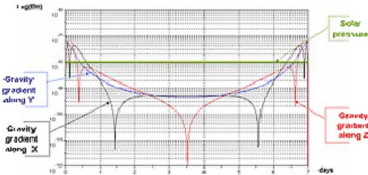
Variation of the gravity gradient on an orbit period along the different axis
