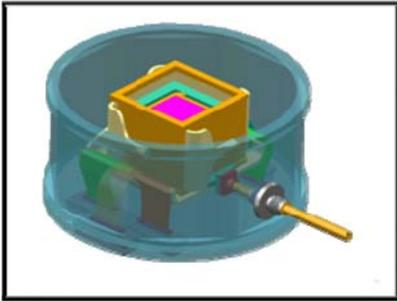
The satellite nuclear noise will be measured and taken into account thanks to an active anticoincidence system which surrounds the detection payload.
