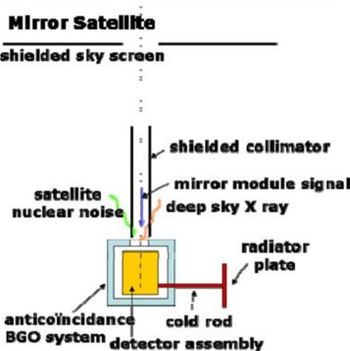
For the deep sky X-ray background a shielded collimator is foreseen. A sharing was to be done on the protections between both satellites. The “mirror satellite” can use a shielded sky screen which blocks the X-rays and the “detector satellite” uses a collimator.
