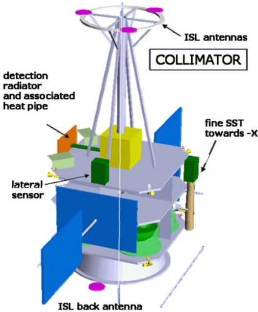
On the following scheme showing details of the propulsion system, the collimator crosses the whole platform.
