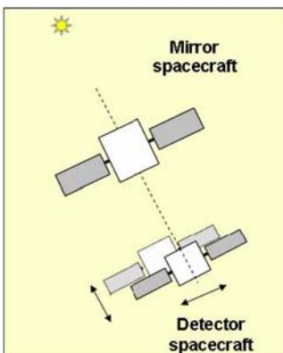
Formation guidance is located by choice on the detector spacecraft which directly communicates with the Ground Station. This strategy is still to be confirmed but by this way during routine science phases the formation could be seen by the Ground Segment as a
