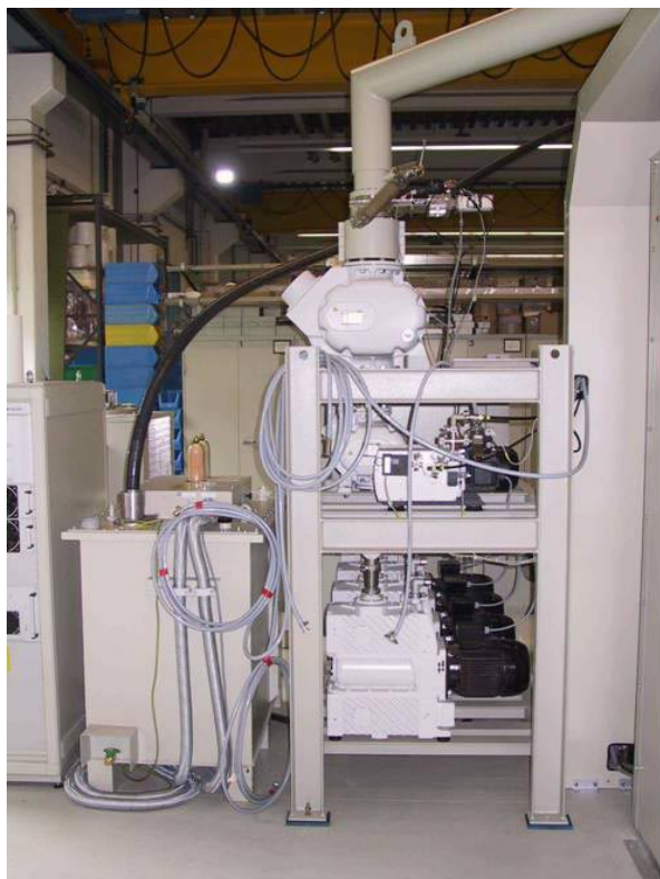
Fig.JRA1.2.7: Oil free fine vacuum pumping station
