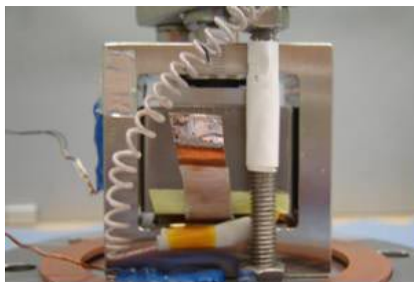
Fig.JRA1.8.3 Sample of magnetostrictive tuner
