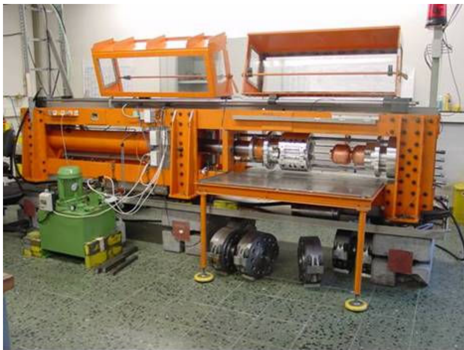
Figure JRA1.3.5: View of the hydroforming machine
