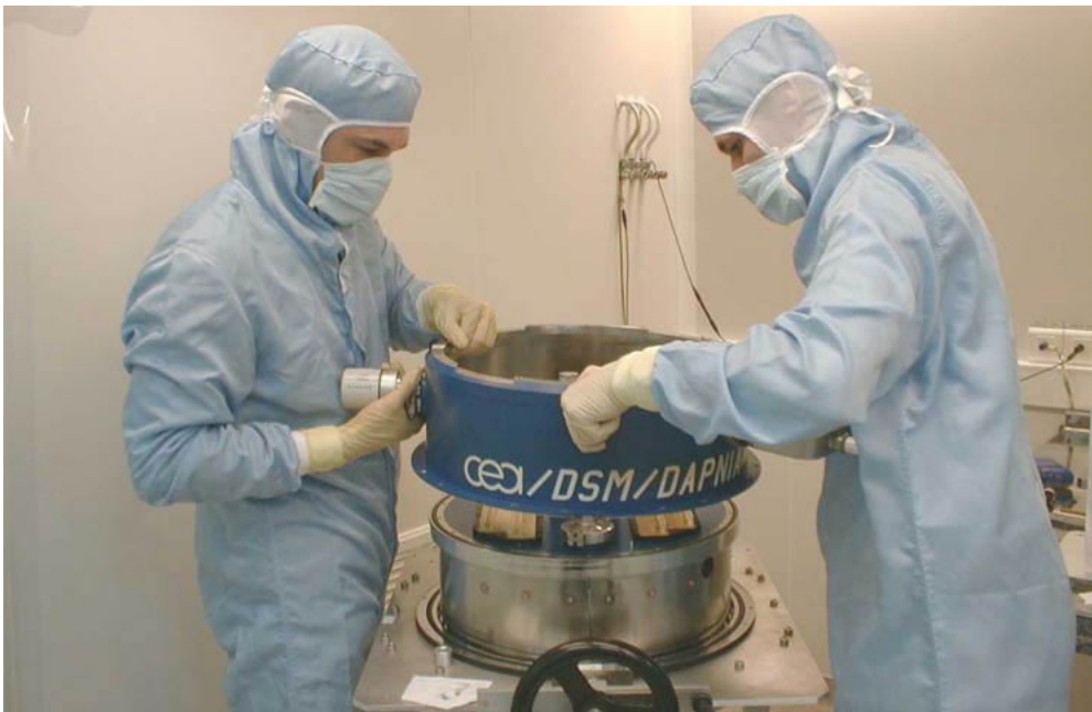
figure 13. Lowering of the cryostat body in the class 100 clean room.
