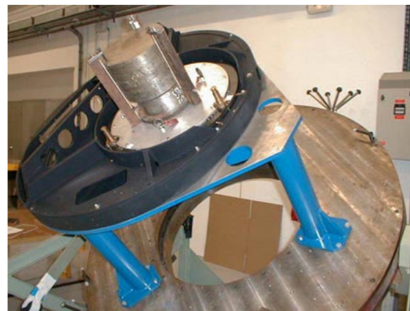
figure 4. Camembert Deformations test on a tilt table
