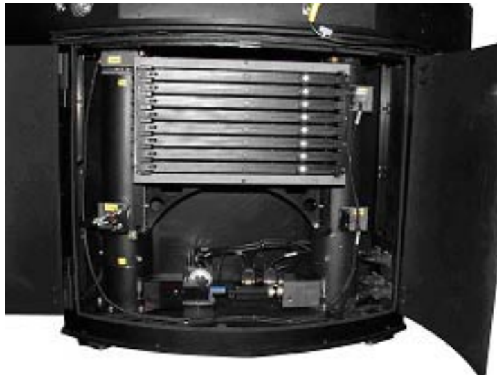
figure 15. View of the jukebox with 8 filters
