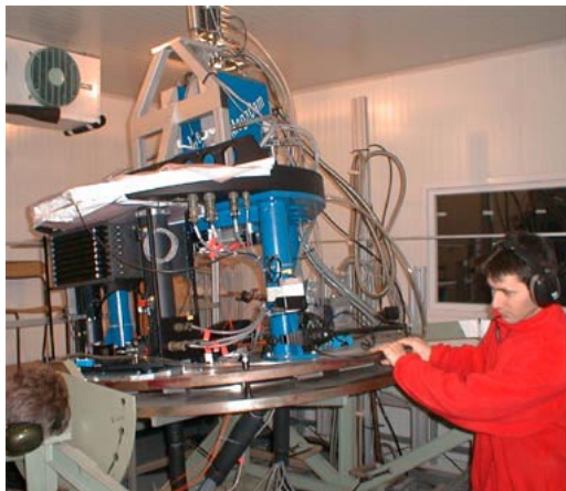
figure 6. Instrument Deformations test on a tilt table and Optical sensor under the CCDs mosaic
