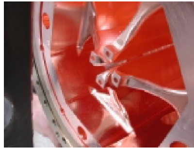
Figure 14 - Radial matching section of the IPHI RFQ after brazing.
