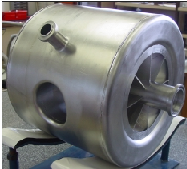
Figure 30 - 352.2 MHz, \beta=0.35 , 2-gap spoke cavity prototype (IPN Orsay – CERCA).
