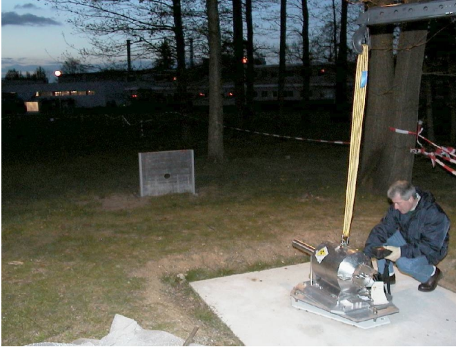
Fig. 7: An artificial gamma ray “star” shines at the Bruyères le Châtel site on April 18, 2001. The ^{24}\text{Na} high activity radioactive source is ready for operation 125 m away from the SPI germanium spectrometer.
