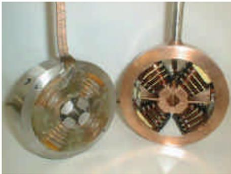
Figure 24 - The magnets manufactured for the DTL short model. Left: Permendur magnet, right: soft iron magnet.
