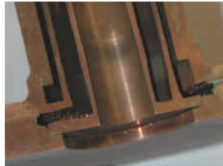
Figure 25 - Test piece of the transparent welding for the AES drift tube (interface between the three concentric stems and the drift tube two-parts body).
