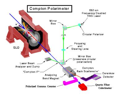
Figure 2. Layout of the SLD Compton Polarimeter at SLAC. Three types of particle detectors were used: Cerenkov counter for electrons, calorimeter, polarized  $\gamma$  counter.
