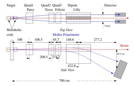
Figure 1. Experimental setup of the JLab Hall A double arm Möller polarimeter.
