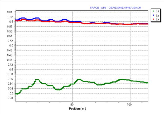
Figure 6: Rms norm. emittances for  $a=4$  and  $q=0.99$ .
