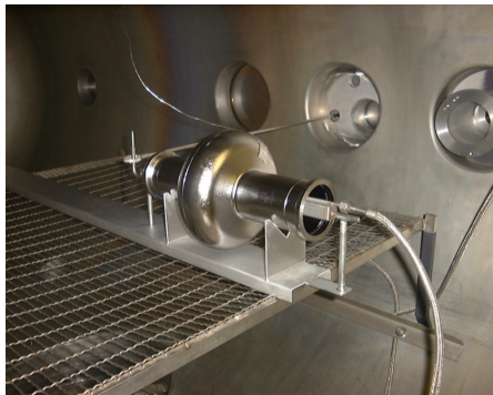
Figure 3: Internal view of plasma reactor with cavity, permanent magnets and gas inlet system.
