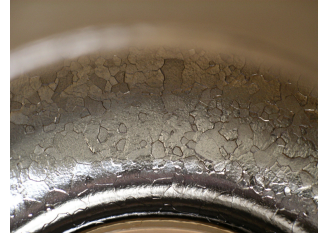
Figure 7b: Picture of the inner surface of C1-15 (no residual Q-slope after baking)
