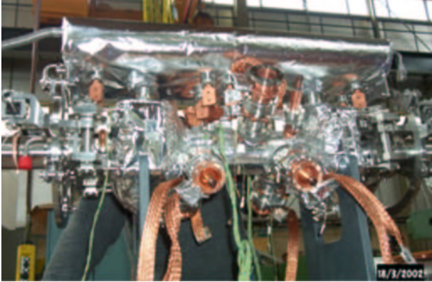
Figure 8: cold mass assembling in the workshop.
