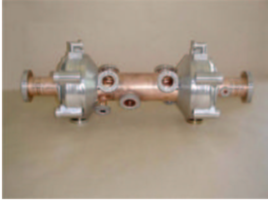
Figure 4: Super-3HC cavity with 2 separate stainless steel helium tanks around the cells.
