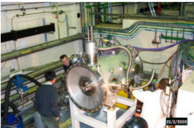
Figure 9: preparation of cryogenic and RF tests of the cryomodule at Saclay before delivery to the machine.
