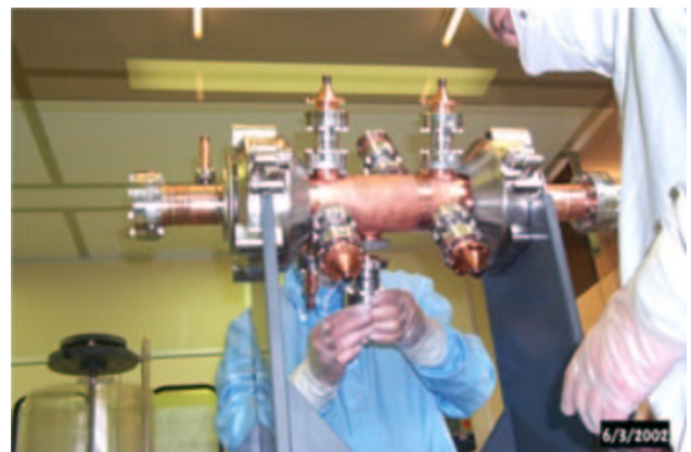
Figure 7: Super-3HC cavity assembling in clean room at Saclay
