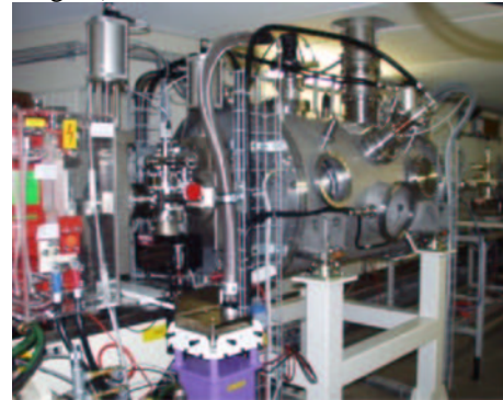
Figure 10: the cryomodule on SLS storage ring.
