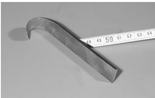
Fig. 5. End spacer machined from copper-aluminum alloy
