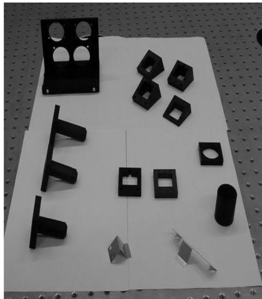
Fig. 9: This picture shows most of the mechanical pieces needed to build a praxial sensor. To ensure the quality of the assembly all elements are screwed and glued on the mechanical support (top left of this picture). The optical elements and their plastic covers are not shown. The assembly of the 2010 praxial elements has started in April 2003. The calibration of all praxial elements will take 17 months.
