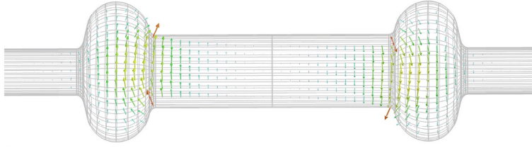
Figure 4: Electric field ( yz ) plane, second dipole mode
