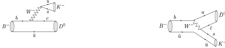
Figure 8: Feynman diagrams for B^- \rightarrow D^0 K^- and B^- \rightarrow \bar{D}^0 K^- . The latter is CKM and color-suppressed with respect to the former.
