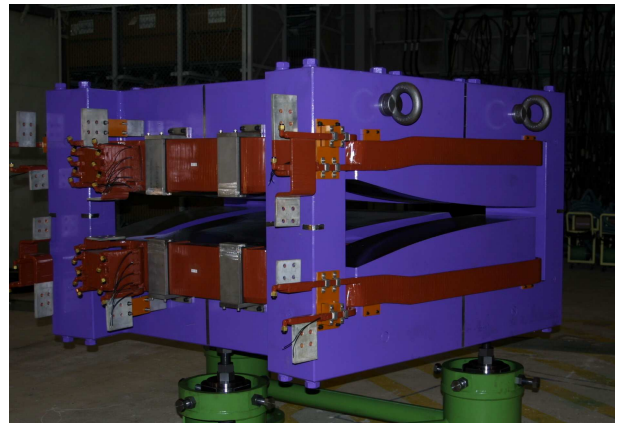
Figure 2: The 150 MeV FFAG DFD triplet. The theoretical field law in the dipoles is of the form B(r) = B_0(r/r_0)^k with B_0 the field at some reference radius r_0 .
