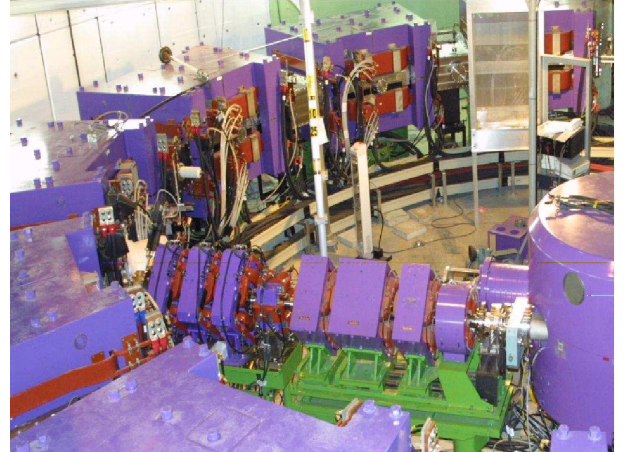
Figure 1: A view of the FFAG ring and of the injection cyclotron and 12 MeV line.
