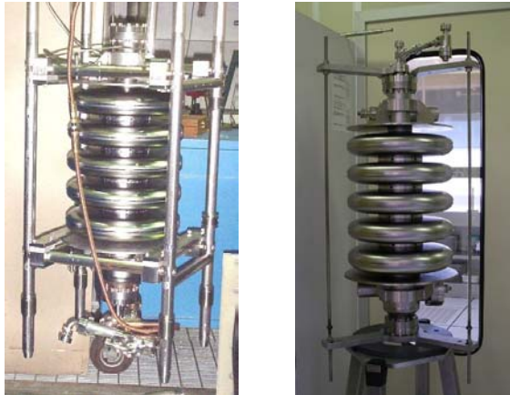
Figure 2: The cavity supports at TJNAF (left) and at Saclay (right).
