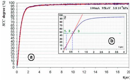
Figure 2: SCC of a rigid beam at 3.8 · 10<sup>-4</sup> hPa.
