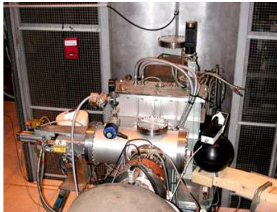
Figure 2 : picture of the probe installation on the beam line.
