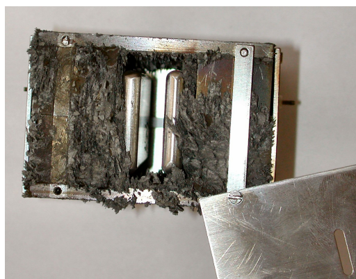
Figure 12 : Picture of the exploded permanent magnet.
