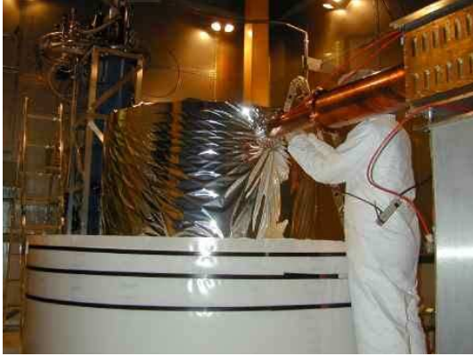
Fig. 17. Setup of the CDMS-II experiment in the Soudan underground laboratory (Minnesota). The cold box, made of ultrapure copper, is surrounded by a passive polyethylen shielding against neutrons from the rock and concrete. An external lead shield is used as a further protection against the gamma-ray background. In the Soudan laboratory, the muon flux is reduced by a factor \sim 10^5 compared to ground level, but a muon veto (not shown on the photograph) is used to identify the remaining muons or showers crossing the detector setup
