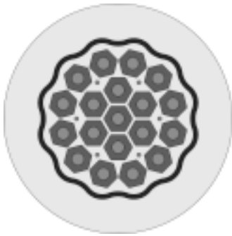
Fig. 5: Example of FE model for mechanical analysis of internal tin wires (Cu is represented in light grey, Ta in black and Sn in medium grey; the multifilament areas surrounding each tin pool, made up of 200 Nb rods in a pure Cu matrix, are represented in dark grey by an average material).
