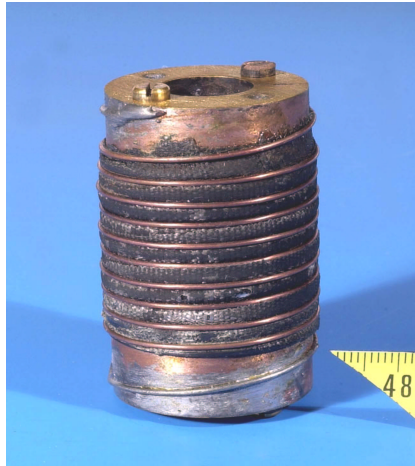
FIGURE 8. Vamas coil for J_c measurement; the pre-impregnated tape wraps the cylinder.
