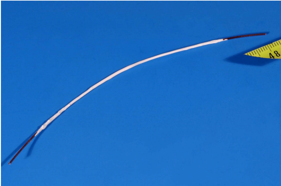
FIGURE 6. Nb 3 Sn wire covered with ceramic solution for RRR measurement.
