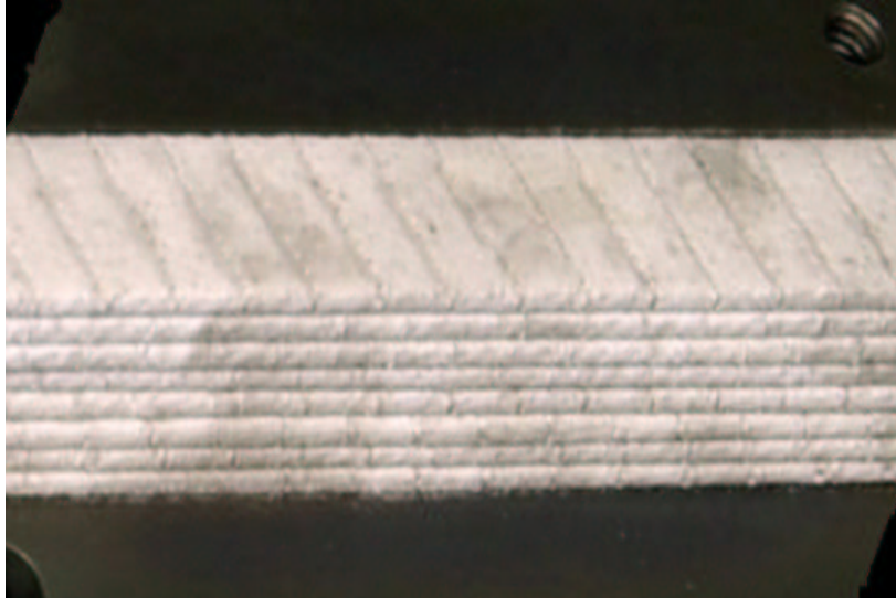
FIGURE 5. Stack of Nb 3 Sn cables insulated after heat treatment, which present a good cohesion.
