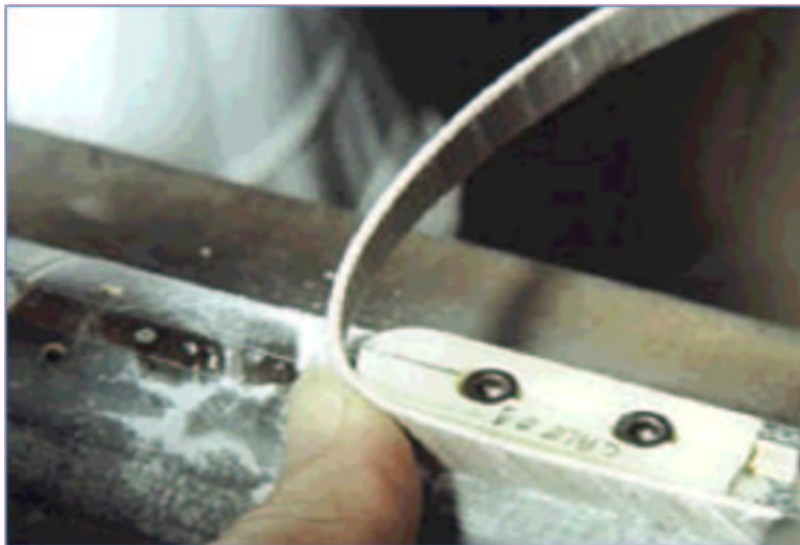
FIGURE 4. Bending test on un-reacted \text{Nb}_3\text{Sn} cable wrapped with impregnated ribbon.
