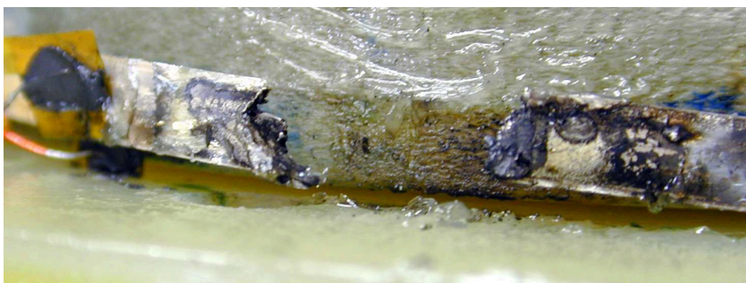
Figure VI.5: Local destruction of a Bi-2212 tape. The sample and the strain gage burnt out before the normal zone expands inside the superconductor. The order of magnitude of the energy necessary to trigger a transition was of tens of Joules at most.
