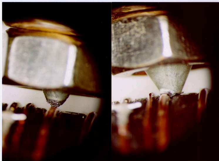
Figure III.6: Zoomed views of the tip of heater 2: left, the heater is simply positioned and no pressure is applied ; right, the heater, at its final position (strongly pressed onto the sample), does not fully cover the sample despite its large contact area compared to the sample.
