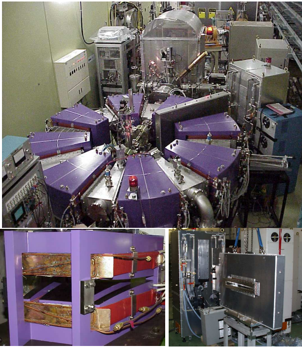
Figure 4: POP FFAG, FDF dipole triplet with scaling gap, broad band accelerating cavity.
