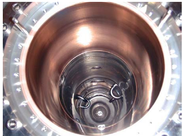
Figure 1: What the electron beam can see when entering the SOLEIL cavities
