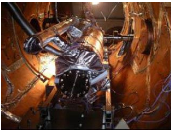
Figure 5: Nine-cell cavity in CryHoLab with high power coupler.
