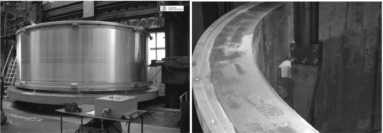
Fig. 3 The large lathe; (a).the machining of the outer surface of a mandrel; (b) the machining of the inner surface of a finite module for removing resin excesses. This latter is a very critical operation since the proximity to the winding (1 mm ground insulation)
