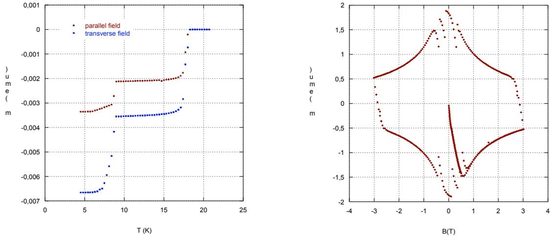
Figure 2: Magnetization measurements on SMI/NED wire: (a) as a function of temperature (left) and (b) as a function of field (right; courtesy of P. Fabbriatore and M. Greco, INFN-Genoa, C. Ferdeghini, INFN-Genoa and U. Gambardella, INFN-Frascati).
